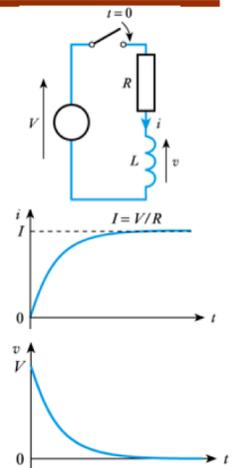
We can perform the same analysis with an inductor being energised (we don't call this charging). At  $t=0$ , when the switch is first closed, NO CURRENT FLOWS, since the current through an inductor cannot change instantaneously. Since no current flows, voltage across the inductor must be  $V$ , the same as the voltage source. Therefore as soon as the switch is closed,  $v$  goes from 0 to  $V$  instantaneously! This is a characteristic of a LR circuit.
