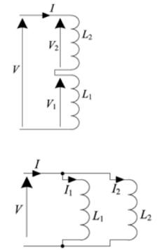
Series and parallel inductors combine just like resistors do.
