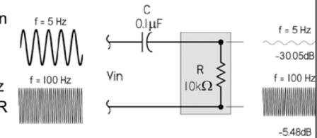
Signal Attenuation vs. Frequency
